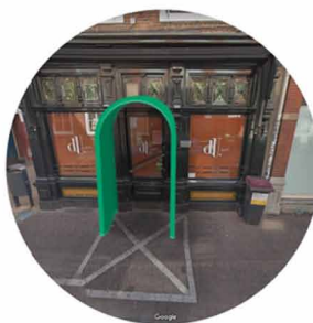
B Sound absorbing tunnel at exit club
